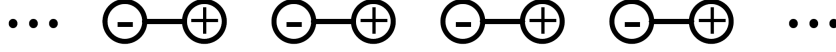
Figure 7.1: As a series of dipoles line up end to end, one can see a current flowing through the line of dipoles as they oscillate back and forth in their polarity. This is similar to how displacement current flows through a capacitor.
